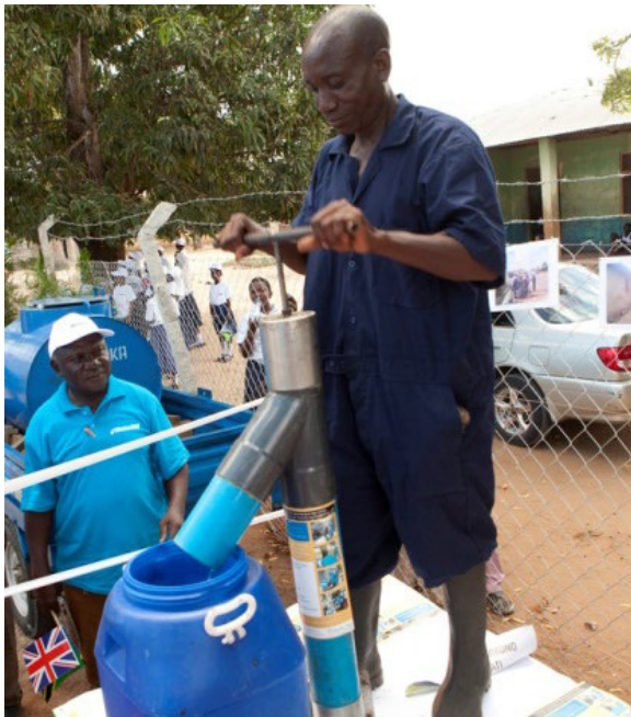
Figure 5.18 Gulper operated desludging
