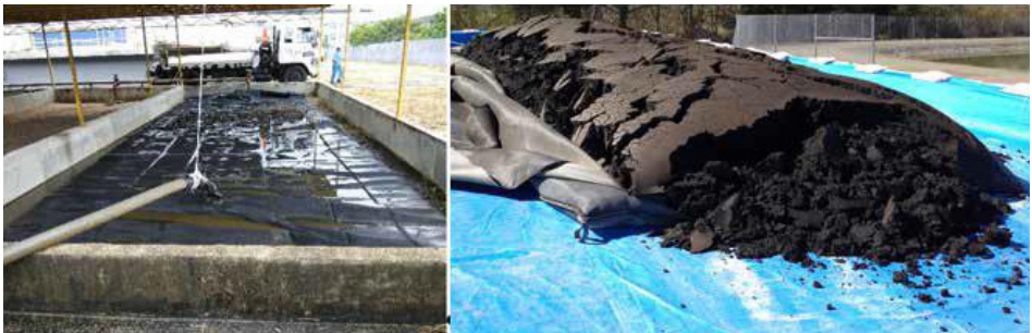
Figure 8.10: Use of Geotubes for Solid Liquid Separation
